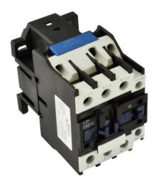
**PART NUMBER – LC1D3210**: Aftermarket direct replacement contactors for Telemecanique LC1D3210, TeSys D Series, type LC1D, 3P, 3PH, 50A, 600V, voltage max 20 hp, 1 N/O auxiliary contact, AC magnetic contactor, suitable for use with LC1-D series motor control systems.
