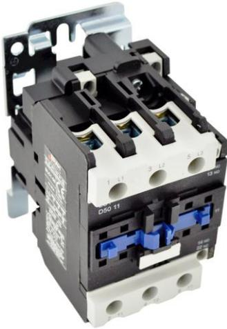
**PART NUMBER – LC1D5011:** Aftermarket direct replacement contactors for Telemecanique LC1D5011, TeSys D Series, type LC1D, 3P, 3PH, 80A, 600V, voltage max 40hp, 1 N/O - 1 N/C auxiliary contact, AC magnetic contactor, suitable for use with LC1-D series motor control systems.
