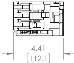
**\*NOTE: BRAH ELECTRIC CONTACTOR LC1D5011 IS AN AFTERMARKET DIRECT REPLACEMENT FOR LC1D5011, LC1-D SERIES. SUITABLE FOR USE WITH LC1-D SERIES MOTOR CONTROL SYSTEMS**
