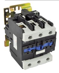
**PART NUMBER – LC1D9511:** Aftermarket direct replacement contactors for Telemecanique LC1D9511, TeSys D Series, type LC1D, 3P, 3PH, 125A, 600V, voltage max 60 hp, 1 N/O - 1 N/C auxiliary contact, AC magnetic contactor, suitable for use with LC1-D series motor control systems.
